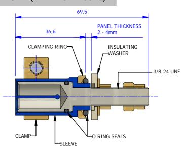
PANEL (BULKHEAD) THICKNESS 2 - 4mm MOUNTING HOLE REQUIRED Ø14.3 ±0.2
